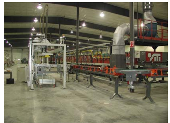
Steuben Tile's main kiln, a custom Siti kiln for continuous firing. Raw Materials batching and mixing facility recently also installed.
