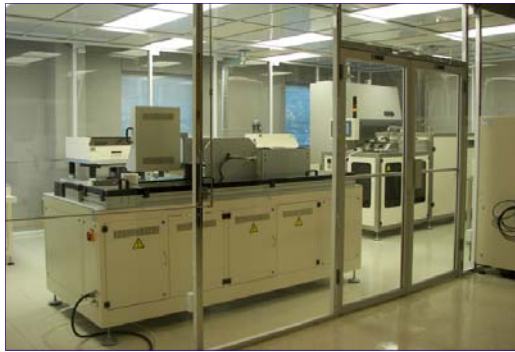
The Class-10,000 cleanroom facility in the new NYSTAR-funded Nanotechnology Pilot Plant in the Alfred Ceramic Corridor Innovation Center.
