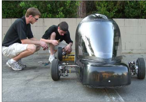
Peifer repositioned the axles to alter weight distribution after test runs on the California course. Total weight (car + driver) was restricted to 350lb.
